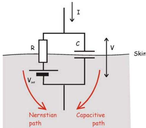
**Figure 3.** Electrode-tissue interface with components representing the ionic to electronic transition phenomena.
