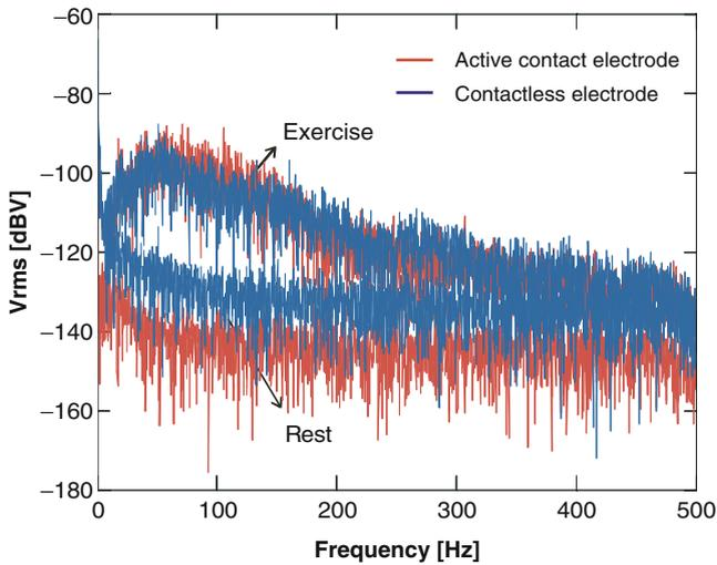
**Figure 8.** Spectra of the recorded EMG signals with both an active- and contactless electrode.
